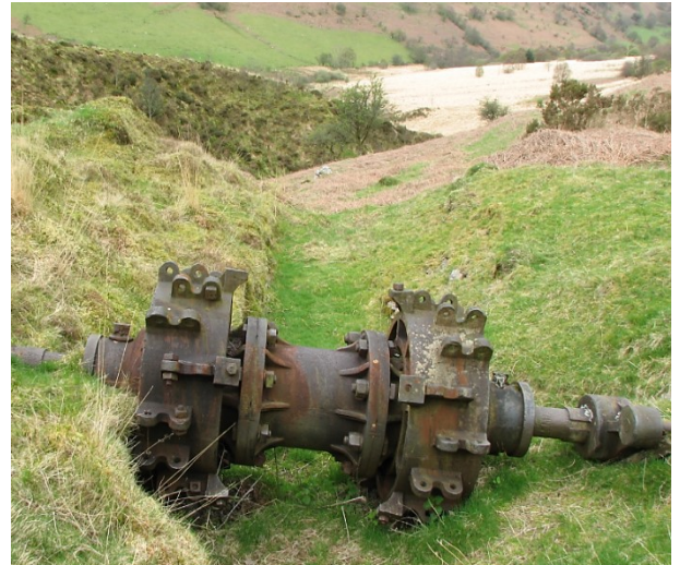
Figure 547: Lead mine at Pistyll y Llyn. (left) Mine shaft. (right) Water wheel pit and remains of the water wheel, installed to pump the mine and lift buckets of ore from the shaft.
